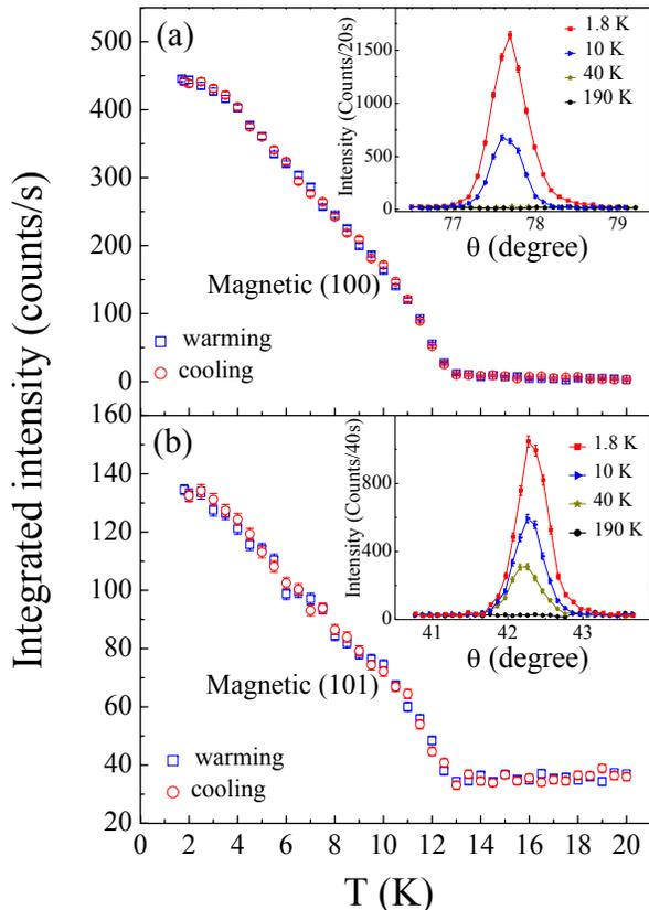
FIG. 3: (color online) Temperature dependence of the neutron integrated intensity for magnetic Bragg peak at (a) (100) and (b) (101). The insets show the corresponding neutron diffraction rocking scans (raw data) at representative temperatures.
