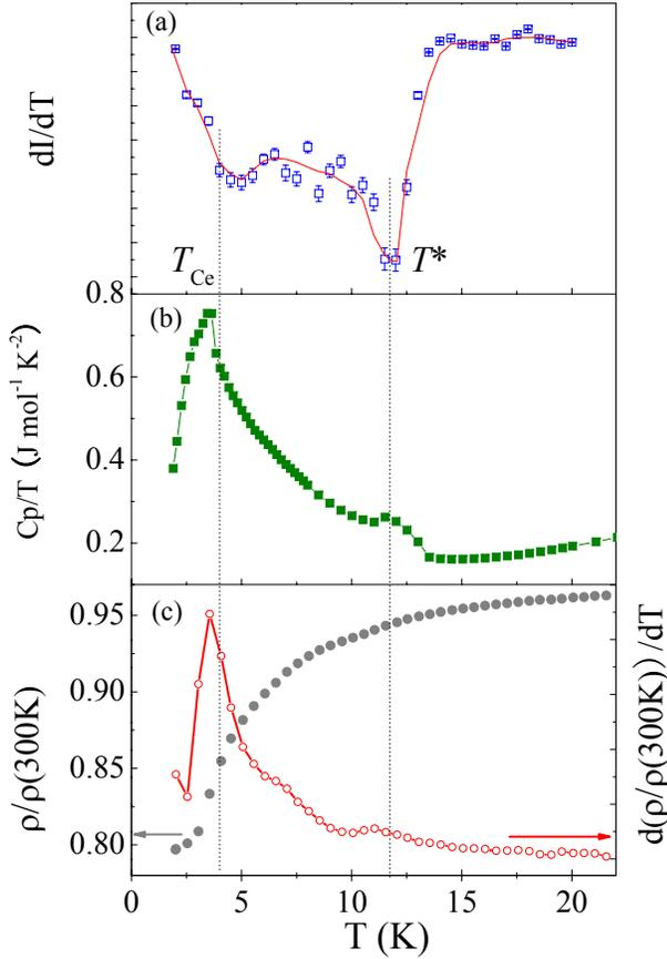
FIG. 4: (color online) Temperature dependence of (a) the first derivative of the neutron integrated intensity for magnetic Bragg peak at (100) (performed numerically), (b) the heat capacity  $C_p/T$  at low temperatures, and (c) the normalized resistivity  $\rho/\rho(300\text{K})$  (left) and its first derivative (right).
