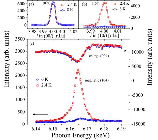
FIG. 6: (color online) Resonant x-ray magnetic scattering at the Ce- $L_{II}$  edge  $L$  scans through (a) charge reflection (004) Bragg reflection and (b) magnetic reflection (104) at 2.4 and 8 K. (c) Photon energy scan at constant- $Q$  values through the Ce  $L_{II}$  resonance at  $T = 2.4$  and 6 K for the strictly charge (004) Bragg reflection and the (104) magnetic Bragg reflection.
