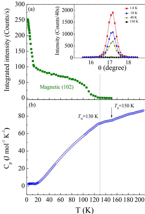
FIG. 1: (color online) Temperature dependence of (a) the neutron integrated intensity of rocking-curve scan of the (102) magnetic Bragg reflection and (b) heat capacity  $C_p$ . The inset of (a) shows the neutron diffraction rocking scans (raw data) through the magnetic Bragg peak (102) at representative temperatures.
