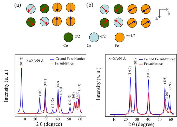
FIG. 10: (color online) (a) The magnetic unit cells of Ce and Fe in polycrystalline CeFeAsO below  $T_{ce}$  proposed by Zhao *et al.* [10]. The bottom figure shows our simulation on the neutron diffraction patterns based on their model. The  $z$  coordinate of Ce is  $\approx 0.1413$ . (b) Our proposed magnetic unit cells of Ce and Fe, and the simulation on corresponding powder neutron diffraction patterns below  $T_{ce}$  in single-crystal CeFeAsO.
