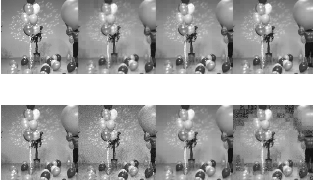
Figure 3: The reconstructed "Balloons" with \sigma^2 = 1e3, \sigma_g^2 = 1e3, \delta = 1/5 . First row (from left to right): original, AMP (PSNR: 27.83dB) , P-GENP-AMP (30.36dB), GENP-AMP (30.42dB). Second row: EMGMAMP-GENP (25.70dB), Residual AMP (18.02dB), Denoising (28.69dB), and Modified CS (14.28dB).
