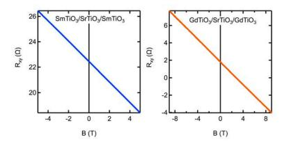
**Figure S2:** Hall resistance,  $R_{xy}$ , ( $\beta = 90^{\circ}$ ) for SmTiO<sub>3</sub>/SrTiO<sub>3</sub>/SmTiO<sub>3</sub> (left) and GdTiO<sub>3</sub>/SrTiO<sub>3</sub>/GdTiO<sub>3</sub> (right) samples, respectively.
