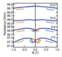
**Figure S1:** Longitudinal magnetoresistance for the GdTiO<sub>3</sub>/SrTiO<sub>3</sub>/GdTiO<sub>3</sub> sample for  $\beta = 0^{\circ}$  and  $\alpha = 0^{\circ}$  as a function of temperature.
