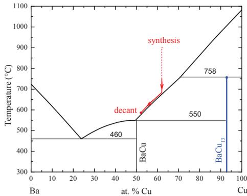
Figure 1: Ba-Cu phase diagram after Okamoto *et al.* [4]. Starting composition and temperature profile for  $\text{Cu}_{13}\text{Ba}$  growths are shown with the red line (the dotted line represents rapid cooling).
