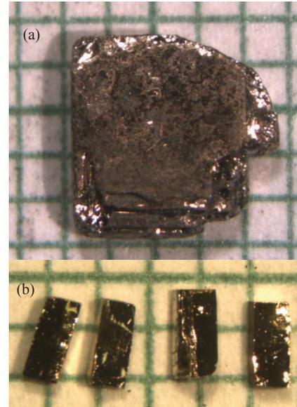
Figure 2: (a) As-grown  $\text{Cu}_{13}\text{Ba}$  single crystal on a millimeter grid. The crystal is 2 mm tall. (b) Single crystals cleaved with a razor blade show a metallic luster and keep it for several hours in air.
