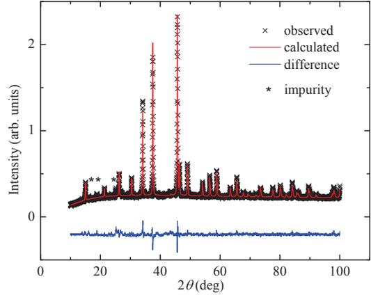
Figure 4: Powder X-ray-diffraction pattern of  $\text{Cu}_{13}\text{Ba}$  with fits based on the published crystal structure. A small amount of an impurity phase, presumably a barium hydroxide hydrate, is inferred from additional peaks marked by asterisks.
