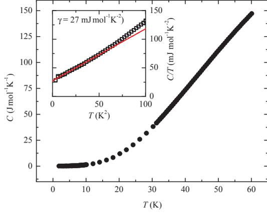
Figure 7: Temperature dependent specific heat of  $\text{Cu}_{13}\text{Ba}$ . The inset shows the linear behavior of  $C/T$  as a function of  $T^2$ , as expected for an ordinary metal, and a Sommerfeld coefficient of  $\gamma = 27 \text{ mJ mol}^{-1} \text{K}^{-2}$  is extracted.
