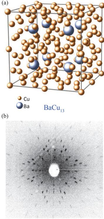
Figure 3: (a) Face-centred cubic unit cell of  $\text{Cu}_{13}\text{Ba}$ . (b) Laue-back-reflection pattern confirming that the single crystals show predominantly  $\{100\}$  faces and cleave along the corresponding planes.
