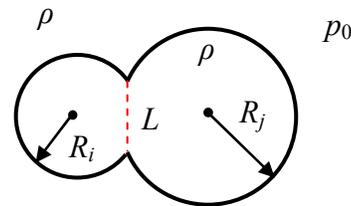
**FIGURE 1.** Cell consists of two connected grains with radius  $R_i$  and  $R_j$  and also intersection length  $L$ .
