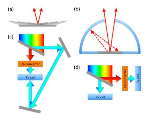
Figure 9. Schematics of possible practical realizations of angular selectivity and spectral splitting in the proposed hybrid converter. Angular selectivity via surface nano-patterning (a) and by enclosing the up-converter into a reflective cavity with a small aperture (b). Geometrical and spectral splitting of sunlight in a configuration with one PV cell (c) and two PV cells (d).
