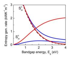
**Figure 8. Entropy generation in the hybrid TPV converter.** The rate of entropy creation in the PV cell  $S_{irr}^c$  and in the up-converter  $S_{irr}^u$  for the ideal hybrid converter with parameters as in Fig. 3 (solid blue), and for the converter with parameters as in Fig. 6a,b and 95/5 level of surface absorptance/emittance characteristics (solid red). The rate of entropy creation in a single-junction PV cell is shown as a dashed grey line for comparison.
