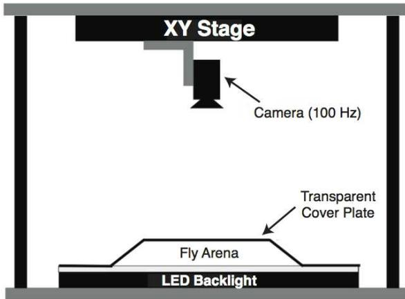
FIG. 1. Schematic of the imaging apparatus.
