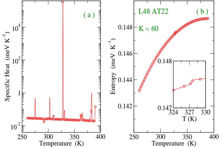
FIG. 4: (Color online) (a) Specific heat and (b) Entropy in the DPB ladder model for the sequence in Eq. (16). The solvent potential is switched off while Morse and stacking potential parameters are as in Fig. 3(a).
