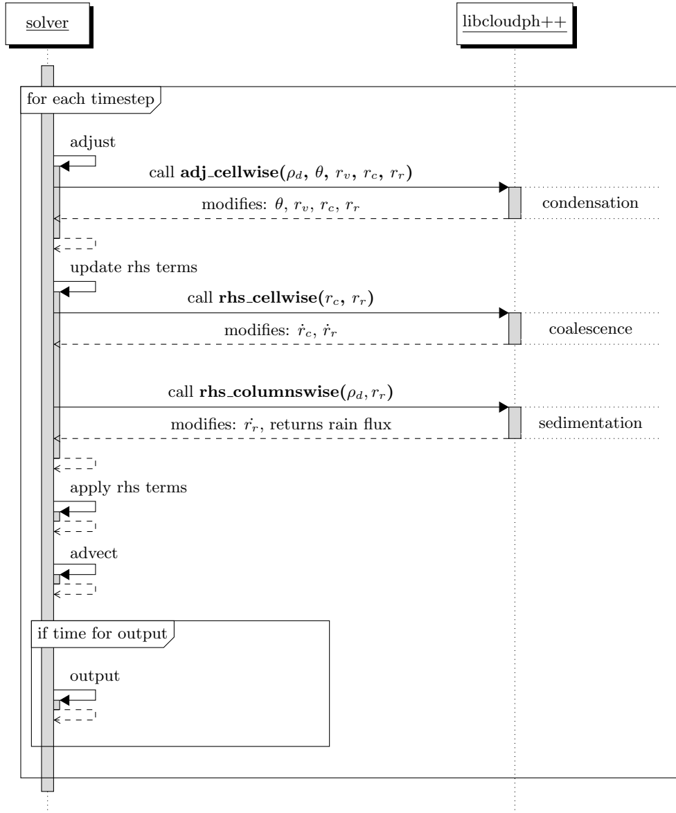
Figure 3: Sequence diagram of libcloudph++ API calls for the single-moment bulk scheme and a prototype transport equation solver. Diagram discussed in section 3.2.2. See also caption of Figure 2 for description or diagram elements.
