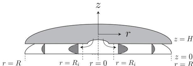
FIG. 3: Schematics of the physical setup to study outward radial flow between two parallel discs. The arrows show the direction of the inlet mass flow. The LBM is used to simulate the flow domain  $0 \leq z \leq H$ ,  $R_i \leq r \leq R$ . We assume that the flow is fully developed for  $r \geq R_i$  and hence the axial velocity  $u_z$  vanishes in this region.
