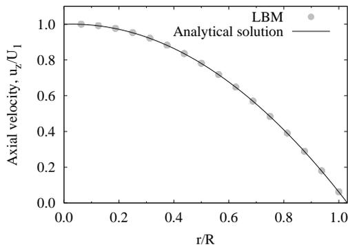
FIG. 2: A comparison of the axial velocity profile as obtained from the LBM simulations (circles) versus the analytical solution (solid line) Eq. (20). Simulation parameters:  $N_z \times N_r = 16 \times 16$ ,  $R = N_r$ ,  $\rho = 1$ ,  $\nu = 0.167$ ,  $g = 10^{-5}$ ,  $U_1 = u_z(0) = 3.84 \times 10^{-3}$ .
