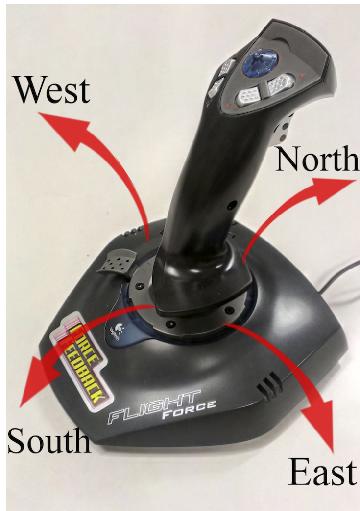
Figure 1. The force-feedback (or tactile-force) joystick FLIGHT FORCE by Logitech used in experiments reported in this paper. The tactile-force stimulus was delivered to the subject's dominant hand. Four movements, defined as North , East , South and West directions, were executed randomly from a computer causing the joystick handle to move and push the subject's hand automatically.
