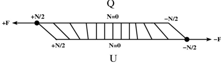
FIG. 4: Schematic representation of dsDNA under a shear force applied at the opposite ends ( $5' - 5'$  or  $3' - 3'$ ).
