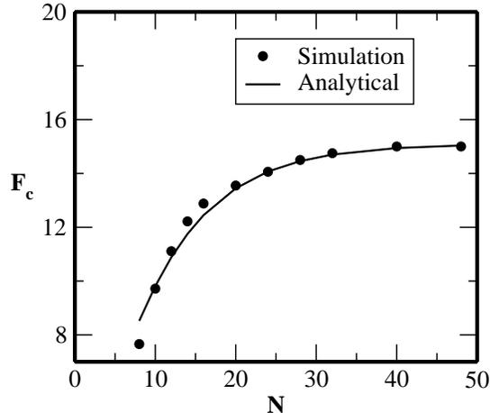
FIG. 6: The variation of rupture force with chain length. The solid line corresponds to a fit of Eq.5 with  $f_1 = 1$  and  $\chi \approx 0.118$ . Solid circles represent the value obtained through the simulation. A nice agreement with the theoretical prediction (Eq. 5) is apparent from the plot.
