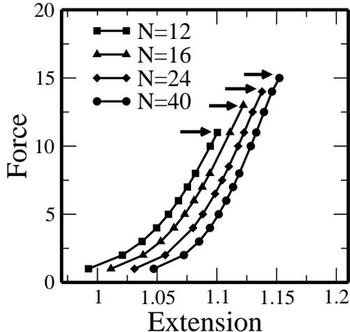
FIG. 5: Force *vs* extension curves for different lengths in the constant force ensemble. Arrows indicate the maximum force, where native contacts approaches to zero and two chains are separated. For the sake of comparison, we have normalized the extension by its chain length.
