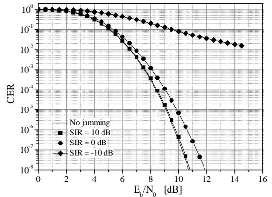
Figure 3. CER performance of the BCH(63, 56) code over CW jamming channel ( $\theta_j = 0$  and  $\Delta\omega = 0$ ), for  $K = 100$ .
