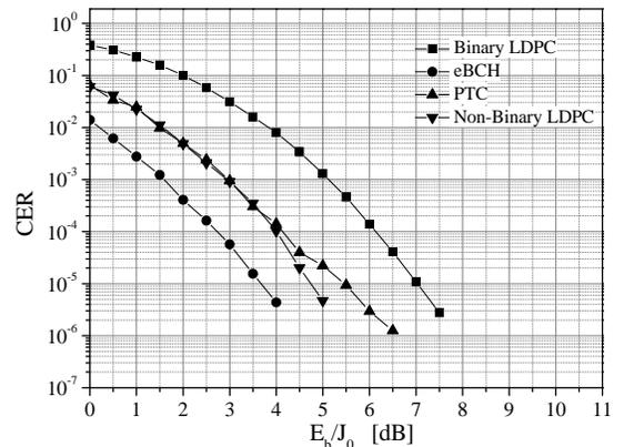
Figure 8. Performance of the new coding schemes ( $n = 128, k = 64$ ) with interleaving and with JSI.
