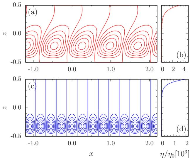
FIG. 8. (color online) Contour lines of the velocity potential  $f$  at the onset of convection corresponding to Fig. 7 for (a)  $\psi = -0.45$ ,  $k_c \cong 4.38$ ,  $R_c \cong 3864$  and (c)  $\psi = -0.55$ ,  $k_c \cong 11.63$ ,  $R_c \cong 5060$ . (b) and (d) depict the corresponding decay of the viscosity.
