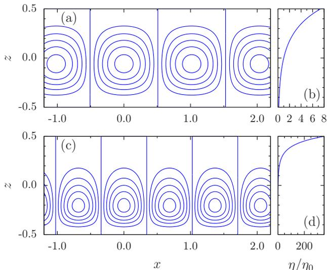
FIG. 2. (color online) Contour lines of the velocity potential  $f$  at the onset of convection for (a)  $\Gamma = 0.002$  and (c)  $\Gamma = 0.008$ , respectively. Parts (b) and (d) show the corresponding spatial dependence of the viscosity  $\eta(z)/\eta_0$ . The critical values are  $k_c = 3.09$  and  $R_c = 1997$  in (a, b) and  $k_c = 4.59$  and  $R_c = 1464$  in (c, d).
