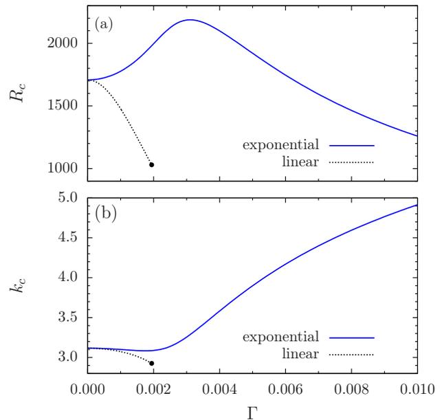
FIG. 1. (color online) (a) The critical Rayleigh number  $R_c$  and (b) the critical wavenumber  $k_c$  for a one-component fluid as a function of  $\Gamma$ . The solid line marks an exponential temperature-dependence of the viscosity, the dotted line represents a linear one. The dotted line ends at  $\Gamma \approx 1.941 \times 10^{-3}$  (black point), where the viscosity becomes negative at the upper boundary.
