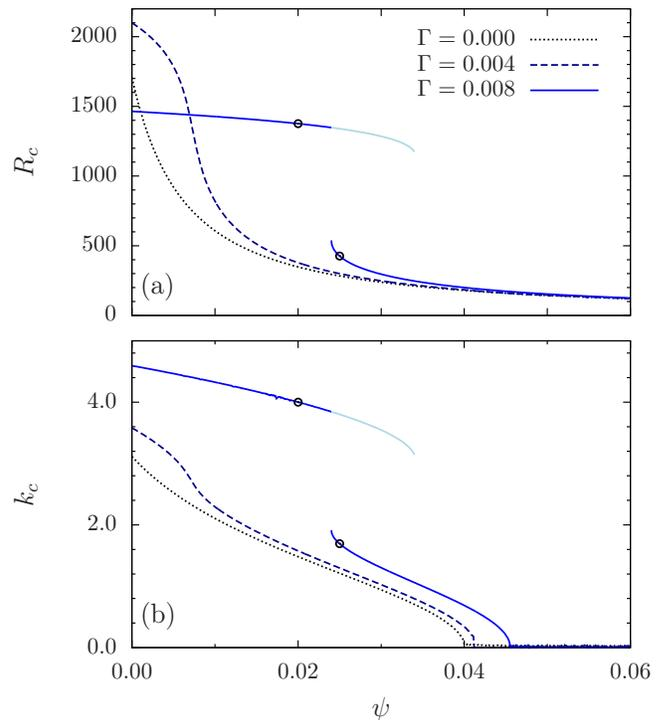
FIG. 3. (color online) Critical values (a)  $R_c(\psi)$  and (b)  $k_c(\psi)$  for  $\Gamma = 0.000, 0.004$ , and  $0.008$ . The circles mark those values of  $\psi$ , for which neutral curves are shown in Fig. 4.
