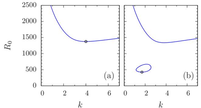
FIG. 4. (color online) Neutral curves corresponding to the circles in Fig. 3 with (a)  $\psi = 0.02$  and (b)  $\psi = 0.025$  for  $\Gamma = 0.008$ . The points mark the minima of the neutral curves.
