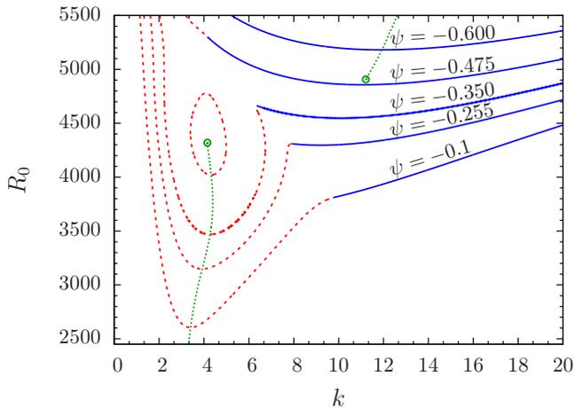
FIG. 7. (color online) Neutral curves for  $\Gamma = 0.003$  and different  $\psi < 0$  as indicated. The green dotted line marks the position of the absolute minima of the neutral curves. The black line denotes the critical value  $\Psi_c \cong -0.5$ , where the transition from an oscillatory to a stationary instability takes place. At that point, the minimum of the neutral curves shows a discontinuous jump in  $k_c$  and  $R_c$  (points).
