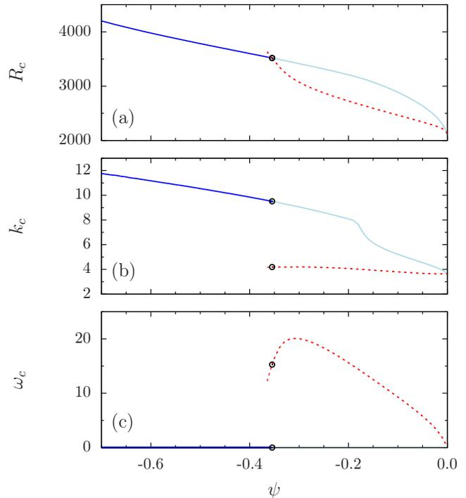
FIG. 9. (color online) (a) Critical Rayleigh number  $R_c$ , (b) critical wavenumber  $k_c$ , and (c) critical frequency  $\omega_c$  as functions of  $\psi < 0$  for  $\Gamma = 0.004$ .
