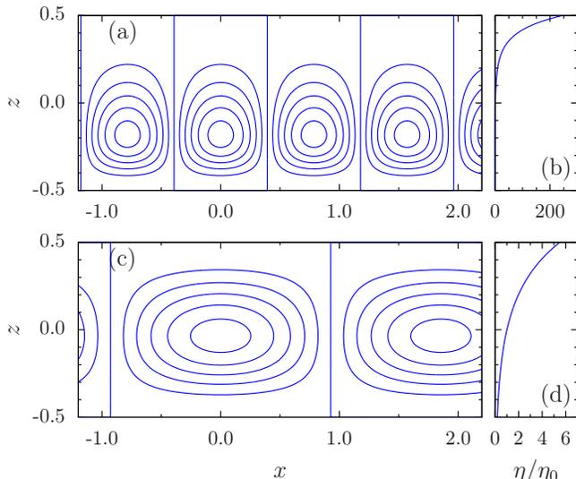
FIG. 5. (color online) Contour lines of the velocity potential  $f$  at the onset of convection corresponding to (a) Fig. 4(a) ( $\psi = 0.020$ ,  $\Gamma = 0.008$ ,  $k_c \cong 4.00$ ,  $R_c \cong 1376$ ) and (c) Fig. 4(b) ( $\psi = 0.025$ ,  $\Gamma = 0.008$ ,  $k_c \cong 1.69$ ,  $R_c \cong 426$ ). (b) and (d) depict the corresponding decay of the viscosity.
