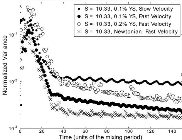
FIG. 2. Variance for different fluids mixed with a stirring ratio of  $S=10.33$ . The same stirring ratio can give different mixing rates based on the rheology of the fluid and the stirring velocity. Representative mixing images are seen in Fig. 1b-d.
