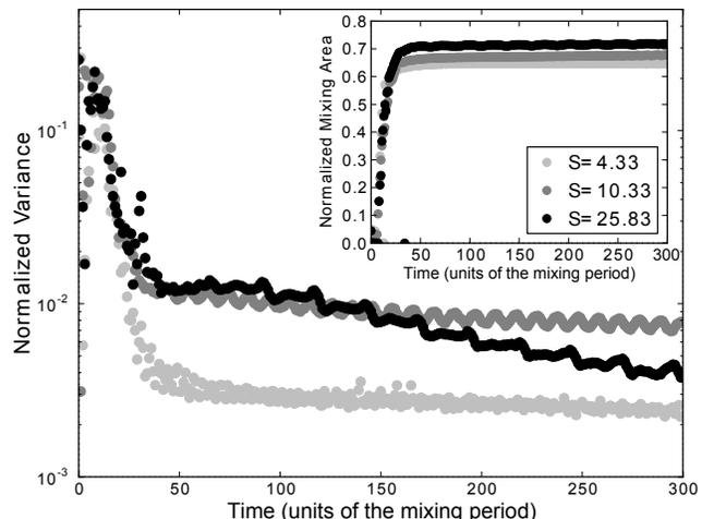
FIG. 3. Mixing rates of 0.1% YS fluid for three different vessel wall speeds, all with a stirring rod period of 6 sec. After the first mixing regime, the smaller  $S$  ratio is the best mixed, but the rate of mixing is higher with larger  $S$  ratios at long time. Inset: mixing area as a fraction of total vessel area for each of the  $S$  ratios. Typical patterns can be seen in Fig. 1d,g,h.
