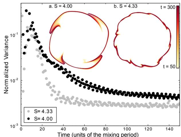
FIG. 4. (Color online) Mixing rates of 0.1% YS fluid for two different vessel wall speeds. Note the slow mixing for  $S = 4.00$  as compared to the  $S = 4.33$  case. Representative mixing images can be seen in Fig. 1f,g. Inset: time evolution of the edge of the mixing area, every 4 rotation periods of the stirring rods, periods ( $t$ ) 50 through 300.
