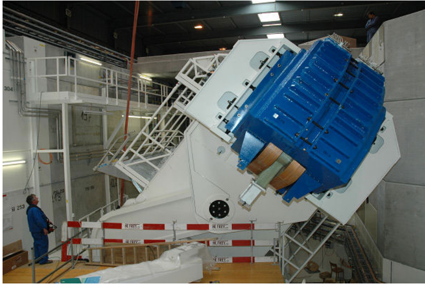
Figure 8: The gantry mechanism and final dipole of Gantry 2 at the Paul Scherrer Institute. The upstream design enables parallel scanning, which thereby simplifies treatment planning and gives an infinite SAD which assists in skin sparing but necessitates a rather large 45-tonne final dipole to give sufficient aperture to deliver the desired treatment field size. (courtesy Prof. Tony Lomax/PSI)
