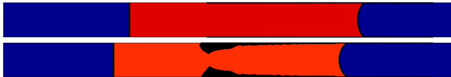
Figure 1: Fluid motion inside an interstice driven by capillary forces. In red the main wetting component, in blue the other substance. The solid phase is represented by black points. The contact angle is the angle that the interface (tangent) forms at the contact line, where the three phases meet. Top: case without surface reaction; bottom: outcome with reaction enabled.
