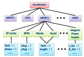
Fig.1: Schematic of the XAL accelerator class hierarchy.
