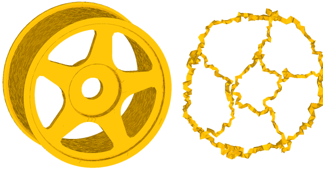
FIGURE 10. A mechanical part and its topology-preserving skeleton.
