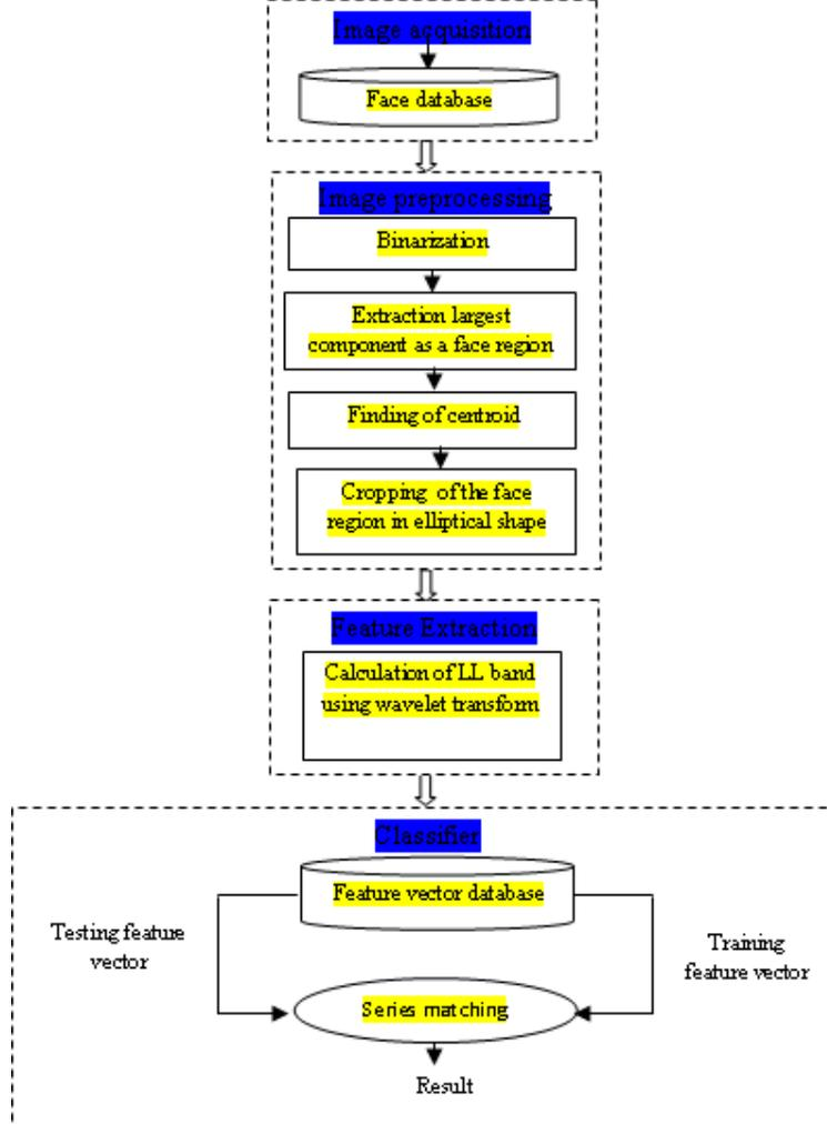
Fig. 1. Schematic block diagram of the proposed system
