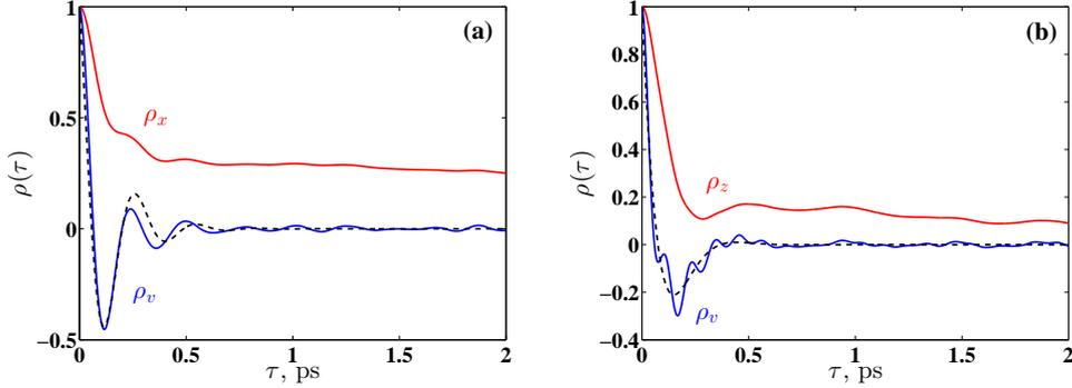
**Fig. 4.** (Colour online) The auto-correlation coefficient of: (a) the coordinate  $x$  (red line) and velocity  $p_x$  (blue line) of the ion in the site S1; and (b) the coordinate  $z$  (red line) and velocity  $p_z$  (blue line) of the ion in the site S0. Dashed lines are approximations of  $\rho_v(\tau)$  by the expression (11).
