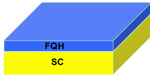
FIG. 1. Schematic setup of a fractional topological superconductor. This state of matter can be achieved by inducing superconducting order parameter into a fractional quantum Hall bar or a fractional Chern insulator through the proximity effect.
