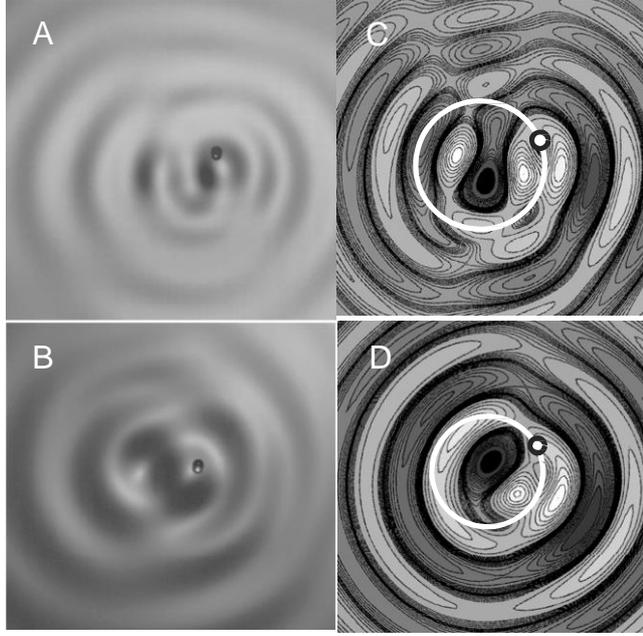
Fig. 4. Comparison of the experimental and computed central regions of the wave field. (A and B) The first two modes  $n = 1$  and  $n = 0$  as observed in the experiment. (C and D) The same orbits obtained in the simulation for a walker with long path memory ( $\tau = 30T_F$  and  $\delta = 1.6\lambda_F$ ).
