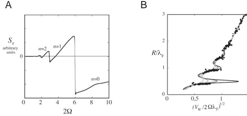
Fig. 6. (A) The variation of the total slope  $S_r(2\pi)$  (of the sources of the last orbit) as a function of the vorticity  $2\Omega$ . (B) The fit of the experimental results by the simplified model (see Eq. 12). Lines are darker for increasing values of the wave amplitude parameter  $A$  in Eq. 12.
