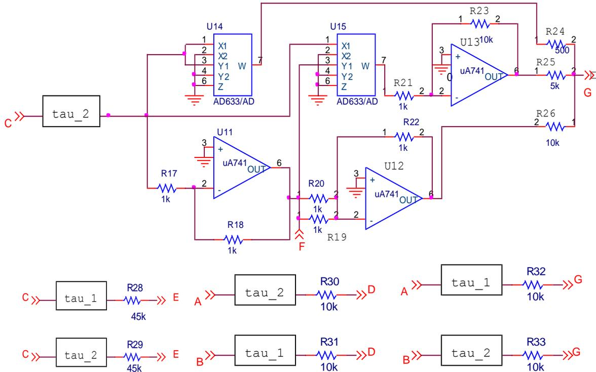
FIG. 4: Delay coupling circuit of the Sprott system. Each of the circuit for  $\tau_i$  ( $i=1, 2, 3$ ) is a LC ladder network where inductor  $L$  and capacitor  $C$  are appropriately chosen to design a desired delay  $\tau$ .
