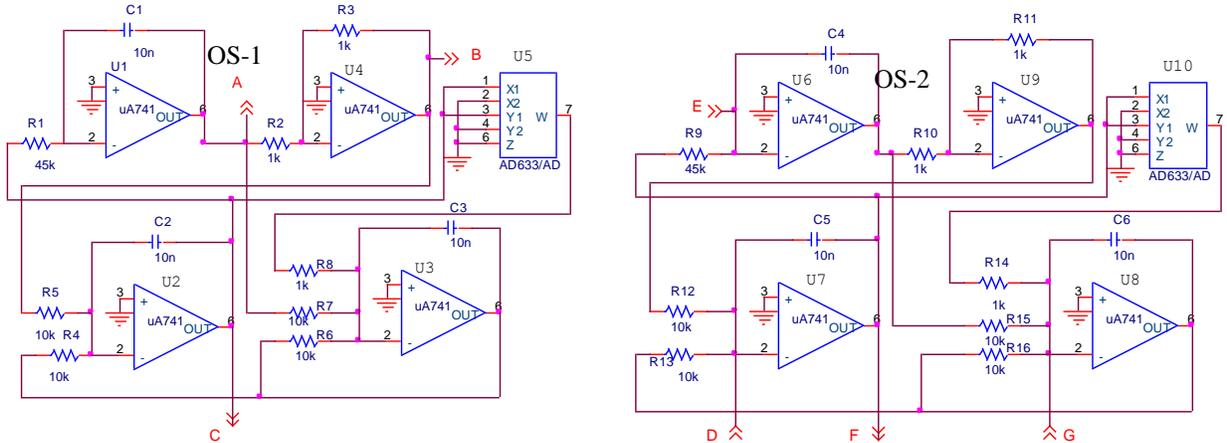
FIG. 3: Circuit of two Sprott systems: driver (left) and response (right) systems. Incoming and out-going connecting nodes (A-G) appropriately connect the delay couplers.
