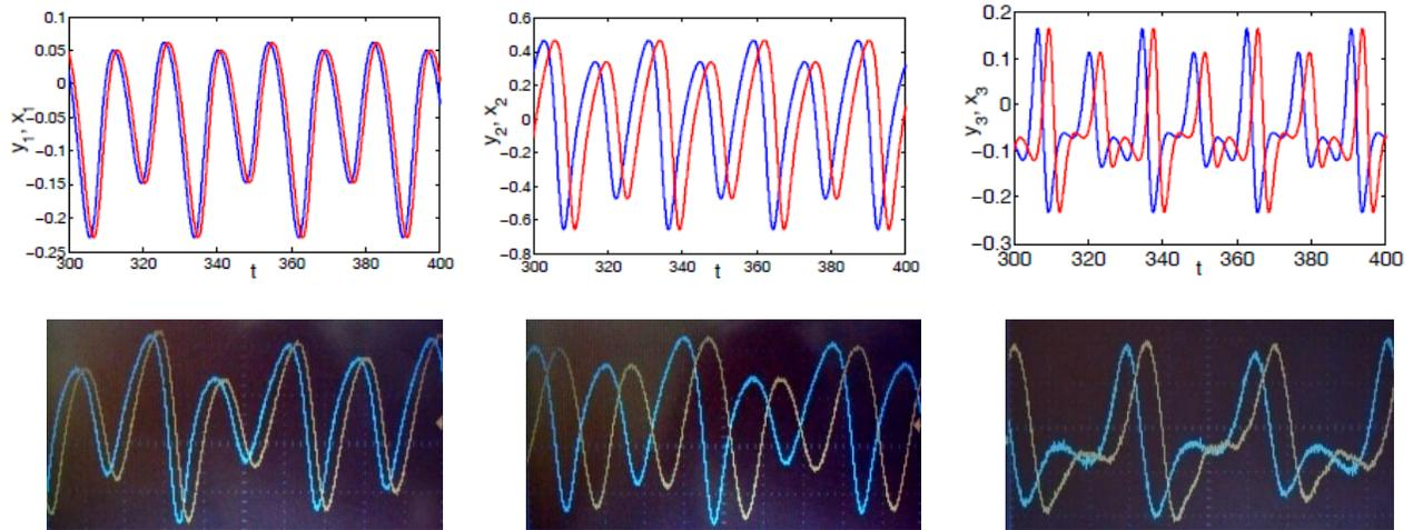
FIG. 5: Numerical and experimental (Oscilloscope picture) time series of the MLS in the upper and lower row. Here  $\tau_1=150 \mu\text{s}$  and  $\tau_2=\tau_3= 400 \mu\text{s}$  for experimental observations and  $\tau_1=1$  and  $\tau_2=\tau_3=3$  for numerical simulations.
