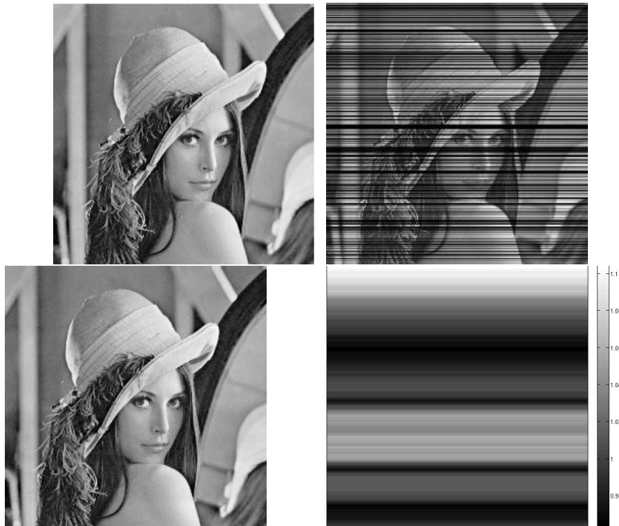
Figure 2: An example involving a multiplicative noise model. From left to right. Original image - Noisy image. It is obtained by multiplying each line of the original image by a uniform random variable in [0.1, 1] . SNR=10.6dB - Denoised using the method proposed in [8] on the logarithm of the noisy image. SNR=29.1dB - Ratio between the original image and the denoised image. The multiplicative factor is retrieved accurately.
