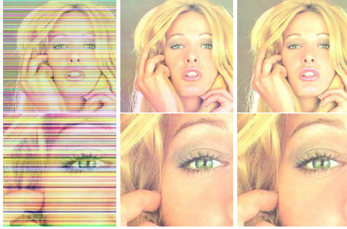
Figure 1: Top: full size images - Bottom: zoom on a small part. From left to right: Noisy image (16,5dB), denoised using the method proposed in [8] (PSNR=32,3dB), original image.
