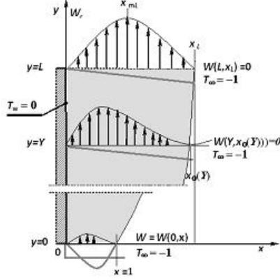
Fig.3 Distributions of velocity and temperature of natural convective fluid flow on characteristic levels of vertical plate  $y = 0, Y$  and  $L$ .
