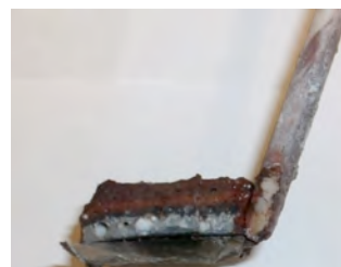
Fig. S-6. Product removed and partially peeled from cathode after 1 or 8 hour electrolyses. The amount of salt removed with the product is high after 1h electrolysis (then washed prior to analysis) & lower after the extended (8h) electrolysis. During the
