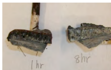
Fig. S-6. Product removed and partially peeled from cathode after 1 or 8 hour electrolyses. The amount of salt removed with the product is high after 1h electrolysis (then washed prior to analysis) & lower after the extended (8h) electrolysis. During the
