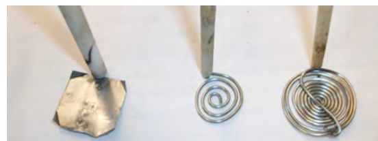
Fig. S-8 (left). Solid steel foil cathodes with various surface areas prior to electrolysis (top) and following electrolysis with partial removal of cathode product (bottom). Spot welds to connect the steel wire contacts are evident.
