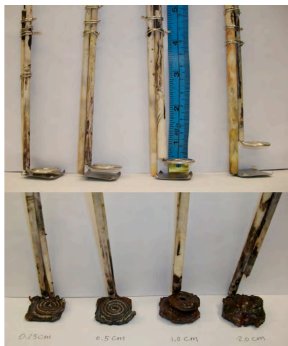
Fig. S-2. Anode (upper electrode) and cathode (lower electrode) prior to electrolysis (top) and following electrolysis prior to removal of cathode product (bottom). Insulating alumina ceramic tubes are reused and hence appear charred.
