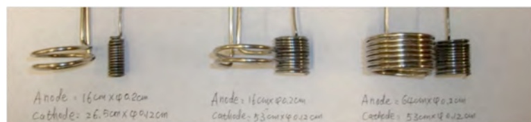
Fig. S-17. Vertical cylindrical configured, coiled electrodes with surface area varied by changing the length and coil diameter of the Ni
