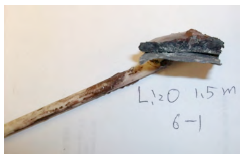
Fig. S-3. Side view of cathode with product.
