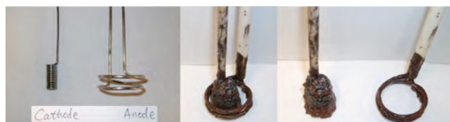
Fig. S-14. Vertical cylindrical configured electrodes used in the molten 730°C lithium carbonate electrolysis in which the cathode was placed inside the anode. Left, middle
