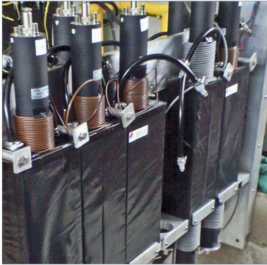
Figure 18: A photograph of the bucking coils on the PMTs of water Čerenkov detectors. A bucking coil of 40 turns was used for each PMT.
