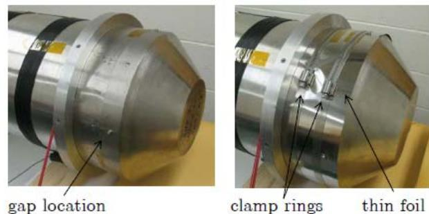
Figure 3: Photographs of the prototype before (left) and after (right) the foil was secured in place with stainless steel clamp rings.
