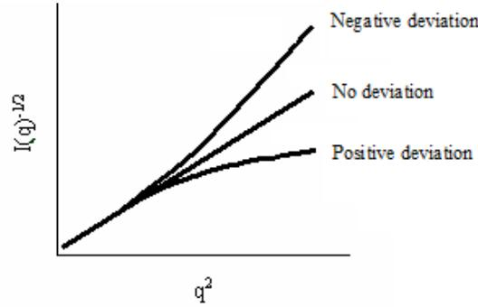
Figure 2 Debye plot with point-collimation in SAXS
