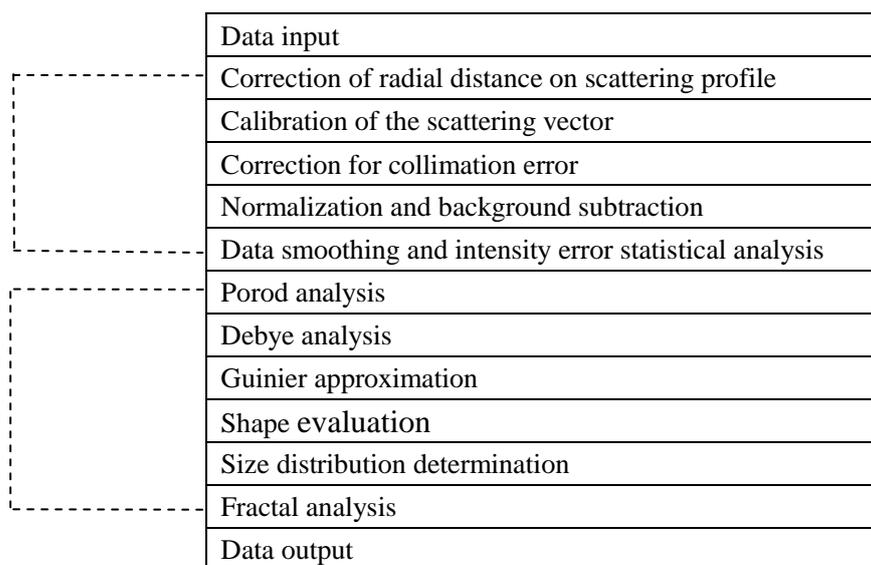
Figure 3 Flow chart of the program S.exe for SAXS data processing and analysis
