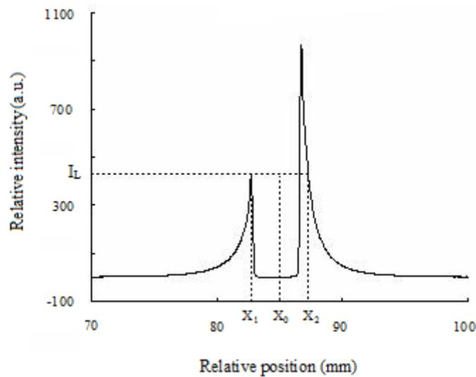
Figure 4 Schematic diagram for correcting the position of direct beam center on an example SAXS profile of a SiO<sub>2</sub> colloid sample
