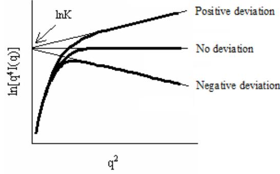
Figure 1 Porod plot with point-collimation in SAXS
