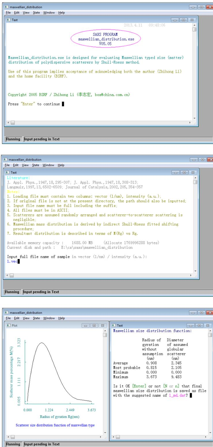
Figure 5: Example of the program execution interface for computation of the scatterers size
