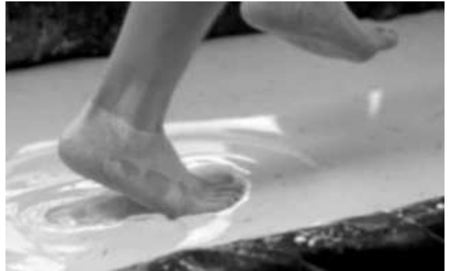
FIG. 1 Snapshot of a person running on top of a pool filled with a dense suspension of cornstarch and water. The fluid can temporarily hold up the person's weight like a solid, sustaining stresses orders of magnitude beyond the capabilities of the suspending Newtonian liquid (here water). The suspension behaves liquid-like before and after impact, for example gravity waves are seen to propagate along the surface, and without running, the person would sink into the suspension as in a normal liquid.
