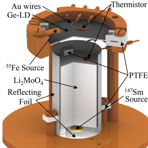
**Figure 1.** Set-up of the detectors. The  $\text{Li}_2\text{MoO}_4$  is held in position by PTFE S-shaped supports. The Ge Light Detector is facing the main crystal in such a way to maximize the light collection. The electrical signals are read from the ground-isolated Cu pins that are connected to the thermistors by means of Au wires.
