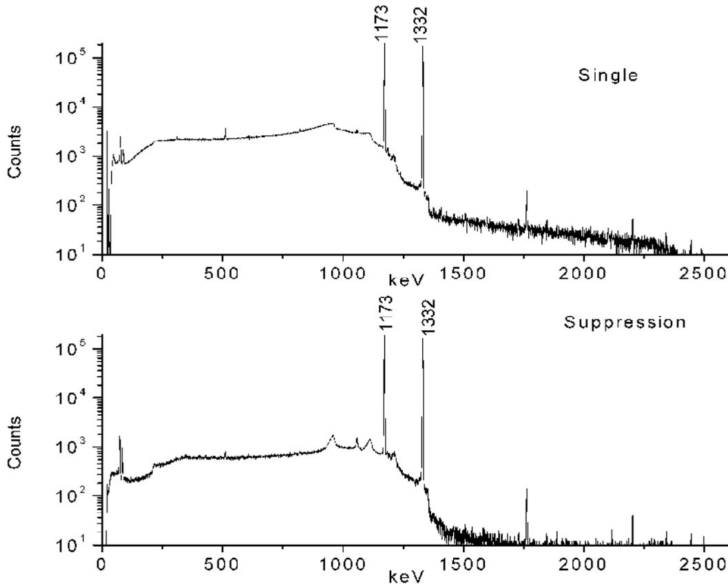
Fig. 4. Single and suppression of  $^{60}\text{Co}$  spectra.
