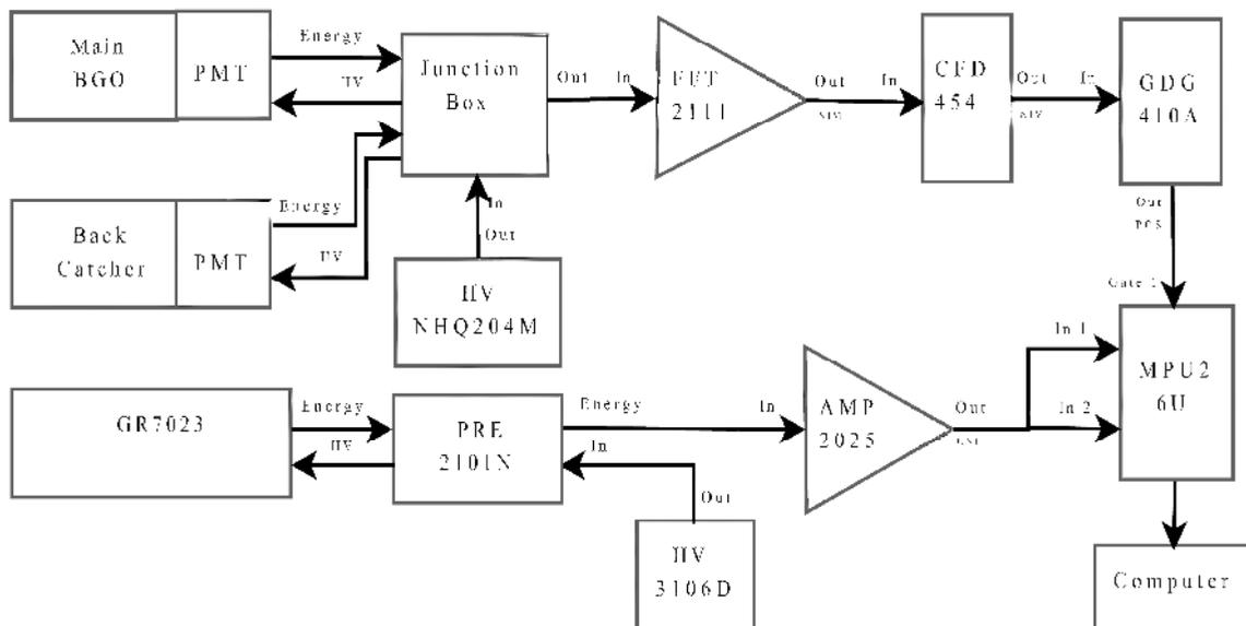
Fig. 1. Configuration of the compton suppression system.
