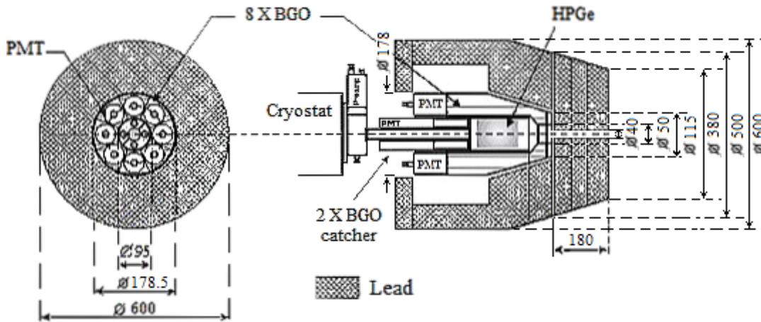
Fig. 2. The back and the cross-sectional view of the detectors and shielding system.
