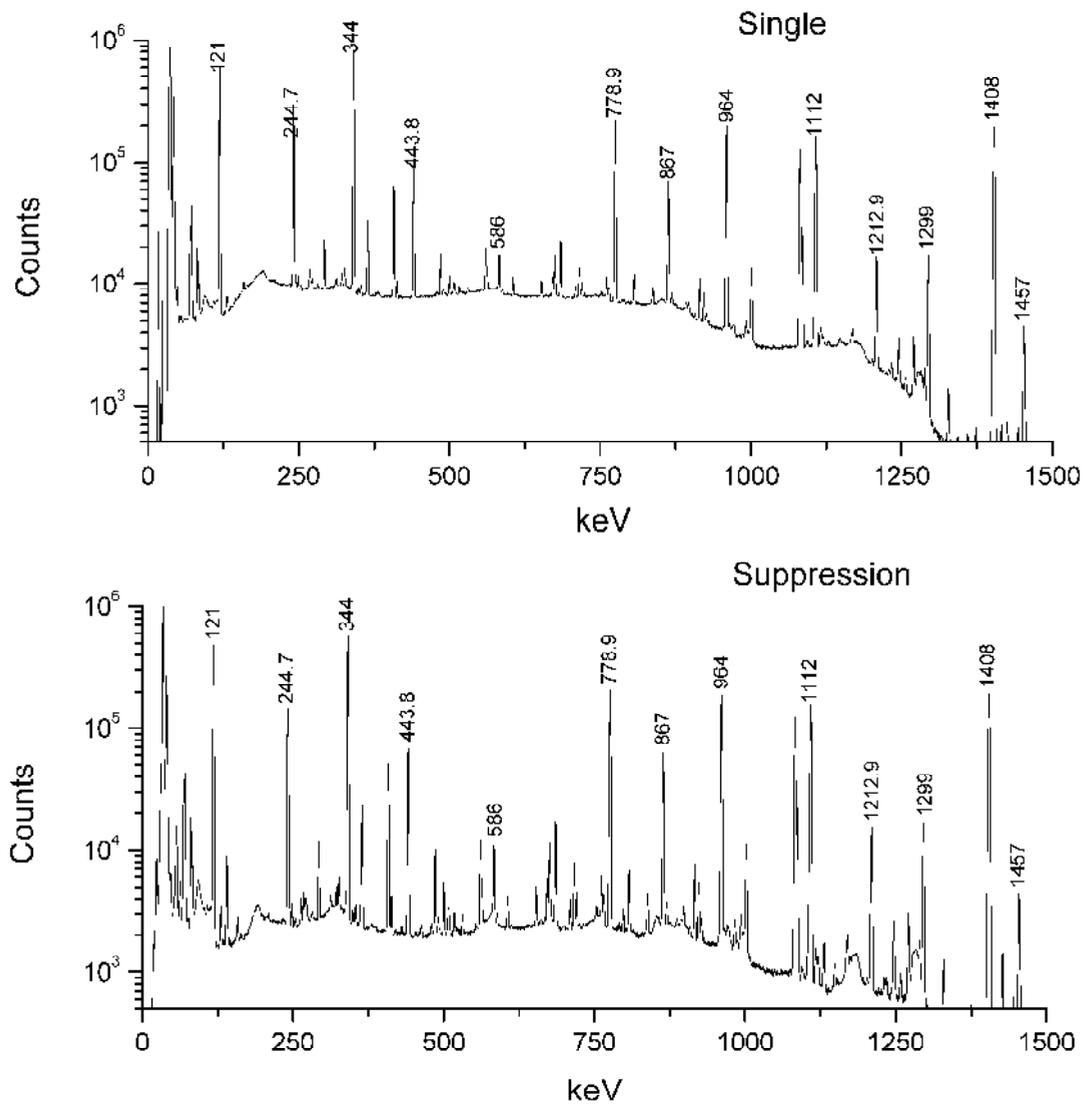
Fig. 5. Single and suppression of  $^{152}\text{Eu}$  spectra.
