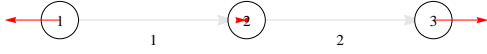
Fig. 2: The gray lines joining the buses show the magnitude of the power flow with the grayscale and the direction of the power flow with the arrows. Each line is numbered as shown. The red arrows at each bus show the oscillation mode shape associated with the critical eigenvalue of the system; that is, the magnitude and direction of the real entries of the right eigenvector x associated to the critical eigenvalue \lambda . 1, 2 and 3 are generator buses.
