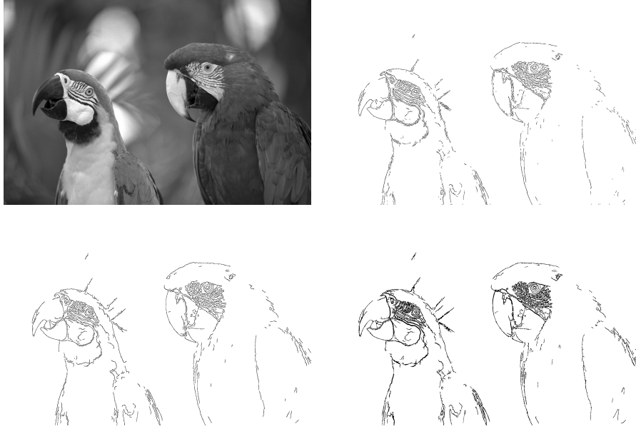
FIGURE 2. Upper left: Original Image. Upper right: Result with Algorithm 1. Lower left: Result with Algorithm 2. Lower right: Result using the Algorithm from [9]. In all examples, the parameters were \alpha = 8 and \beta = 150 .
