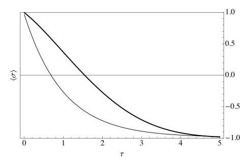
FIG. 1. The denaturing kinetics for a model system. Initially the external conditions make the local free energy difference  $\epsilon = 2k_{\rm B}T$ . At the moment when the scaled time  $\tau = 0$ , the external conditions are suddenly changed so that the local free energy difference abruptly changes into  $\epsilon = -2.5k_{\rm B}T$ . The thinner solid line depicts the case when J = 0, and the thick solid line corresponds to the case in which  $J = 0.5k_{\rm B}T$ .
