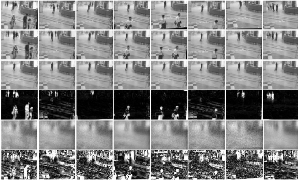
Figure 8: Video background and foreground separation with jittered video. 1 st row: 8 misaligned video frames randomly selected from artificially perturbed images; 2 nd row: images aligned by t-GRASTA; 3 rd row: background recovered by t-GRASTA; 4 th row: foreground separated by t-GRASTA; 5 th row: background recovered by GRASTA; 6 th row: foreground separated by GRASTA.
