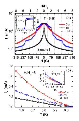
FIG. 2. (Color online) **Critical currents from Sample I.** The magnetic field and temperature dependences of critical currents are presented in (a) and (b), respectively. The inset in (a) shows the zero-field superconducting transitions of the three sections.
