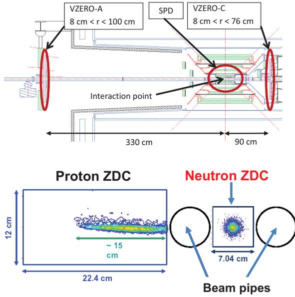
Figure 1: Schematic view showing the approximate positions and shapes of the ALICE VZERO detectors (top) and ZDC detectors (bottom). Top panel: side view of the beam pipe at the ALICE IP. The locations of the VZERO arrays are indicated. Bottom panel: cross section view (perpendicular to the beam line), of the ZDC system.
