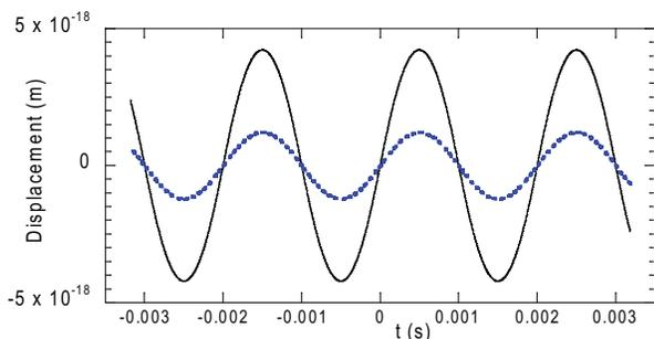
FIG. 1: Steady-state response function  $x(t)$  for deep MOND (solid) and Newtonian (dotted) with the same driving force. A test mass of 16 kg is driven at 500 Hz with a force amplitude of  $2 \times 10^{-10}$  N.
