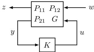
Figure 1: Plant  $P$  connected to a controller  $K$ .
