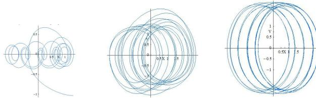
Figure 3: phase diagram : forced Van der Pol generalized oscillator, forced Van der Pol oscillator, and forced Rayleigh oscillator for  $\varepsilon = 10^{-1}$ ,  $E = 1$ ,  $\Omega = 10^{-1}$ .
