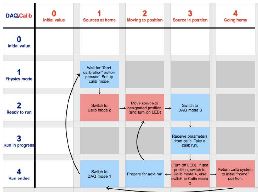
Figure 25: Communication protocol between the control software and DAQ. See text for details.
