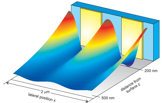
FIG. 1: Sketch of the metal grating including the combined Casimir-Polder and evanescent wave potential landscape as calculated from Eqs. (1) and (2) within Lifshitz theory for a laser power of  $P = 200$  mW. The distances from the surface range from  $z = 200$  nm to  $z = 500$  nm, the lateral position span is  $2 \mu\text{m}$  and the potential modulation at a distance of  $z = 200$  nm is  $\Delta E/k_B = 14 \mu\text{K}$ .
