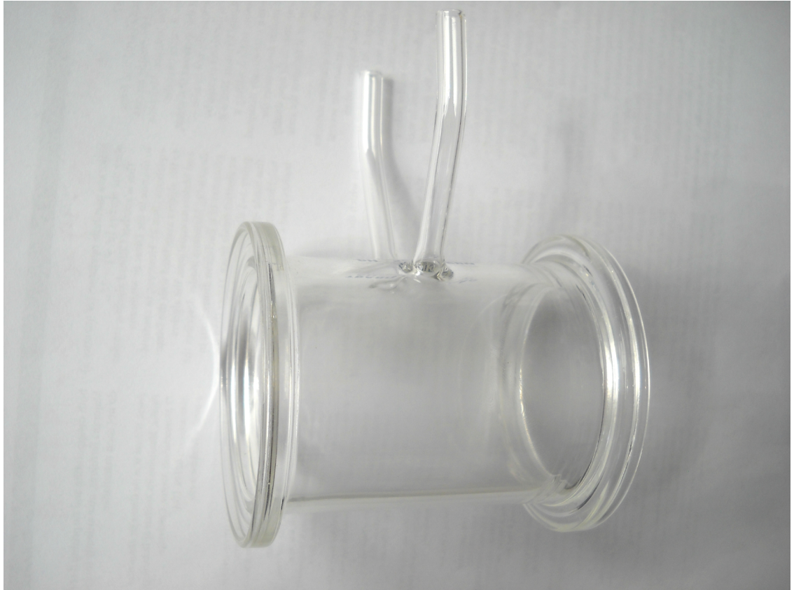
Figure 2. Glass cell used in the setup. O-rings in machined grooves compressed by the quartz plates guarantee vacuum tightness at both ends (not shown on the image). The two glass tubes connecting the cell to the inlet and outlet valve and are coated with Fomblin oil in all measurements.
