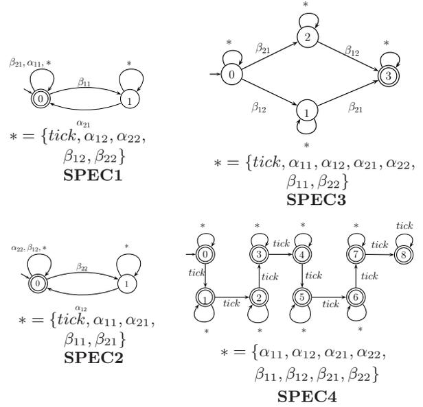
Fig. 6. Control specifications: logical and temporal. The marked state 3 of **SPEC3** corresponds to the completion of a production cycle: one P1-part and one P2-part are processed by both machines.
