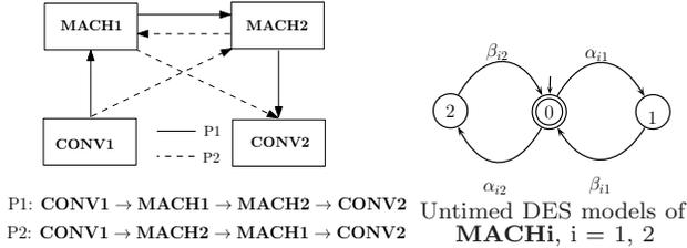
Fig. 5. Manufacturing Cell
