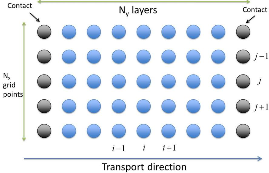
Figure 1: Nano-device partitioned into  $N_y$  layers. Each layer contains  $N_x$  grid points.
