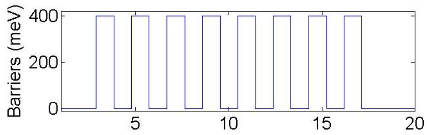
Figure 9: Barrier structure for a model super-lattice device.
