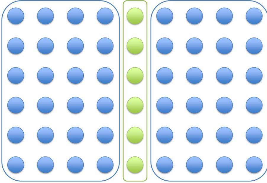
Figure 3: Nanodevice partitioned into two subregions (L, R) and a separator S (L stands for Left and R for Right).
