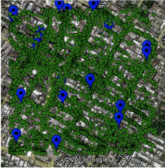
Fig. 2: Google Earth TM map of reported microcell locations (blue balloons) and a fraction of the WiFi sites (green circles) in the East Village, Manhattan. Since the WiFi access points vastly outnumber the current cellular base stations (more than 2000 to 1 in this case), cellular capacity can be significantly increased if femtocells can be co-located at even a small fraction of the WiFi sites.
