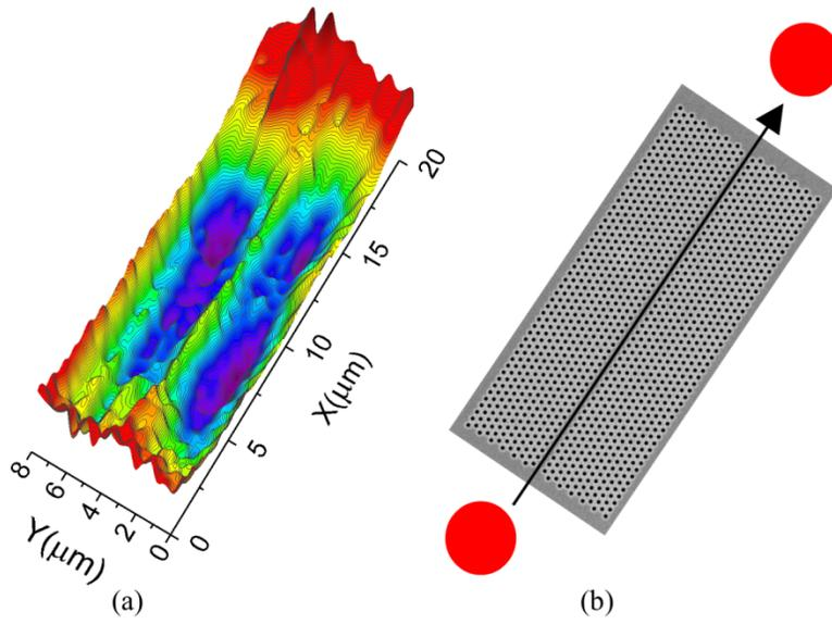
FIG. 2. (Color) (a) Integrated PL mapping of a PhCWG without cavity. (b) SEM image of the PhCWG. The PL mapping is obtained by scanning the laser spot pumping the QDs along the direction of the waveguide defined by the  $X$  axis then translated along the  $Y$  axis.
