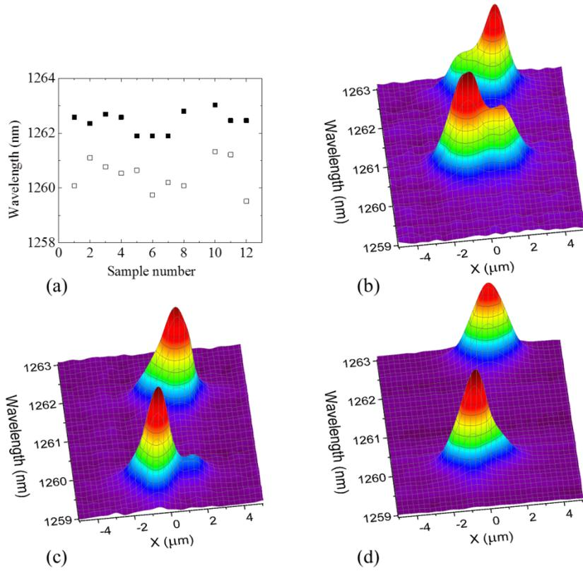
FIG. 4. (Color) Effect of random structural variations in fabricated PMs on the profile of the supermodes of two-coupled PhCWG cavities. (a) High and low energy supermodes of a batch of nominally identical coupled cavity systems measured from the PL spectra. (b-d) PL spectra of coupled cavities obtained along the waveguide direction for each device and presented in increasing order of splitting  $\Delta\Omega = 1.8$  nm, 2.2 nm and 2.8 nm, respectively.
