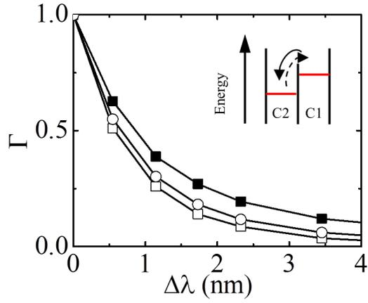
FIG. 7. (Color) Calculated supermode delocalization factor  $\Gamma$  as a function of detuning  $\Delta\lambda$  for two-coupled PhCWG cavities. Results from the semi-analytical approach (circles) are compared with results from the full 3D FDTD on the detuned system for the high (plain squares) and low (empty squares) energy modes. A mechanism to explain the difference between the mode delocalization of the high and low energy modes with detuning is shown schematically in the inset.
