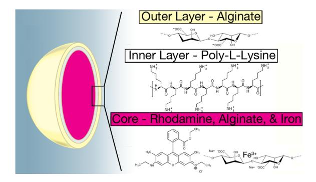
**Scheme 2.** The cartoon shows the APA microsphere composition which includes a central core of Fe<sup>3+</sup>-cross-linked alginate gel loaded with rhodamine 6G dye and a two-layer shell consisting of a poly-L-lysine inner layer and sodium alginate outer layer.
