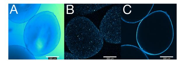
**Figure 1.** Images taken using a confocal optical microscope, where (A) is optical visualization of the microspheres (without fluorescence), (B) is a fluorescent image of the rhodamine-loaded core, and (C) shows a fluorescent image of the FITC-labeled poly-L-lysine outer layer in the shell (note that rhodamine was not included in the core).
